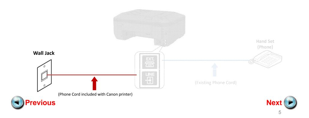
Plug the provided phone cord into the "LINE" jack located on the rear of the multifunction
