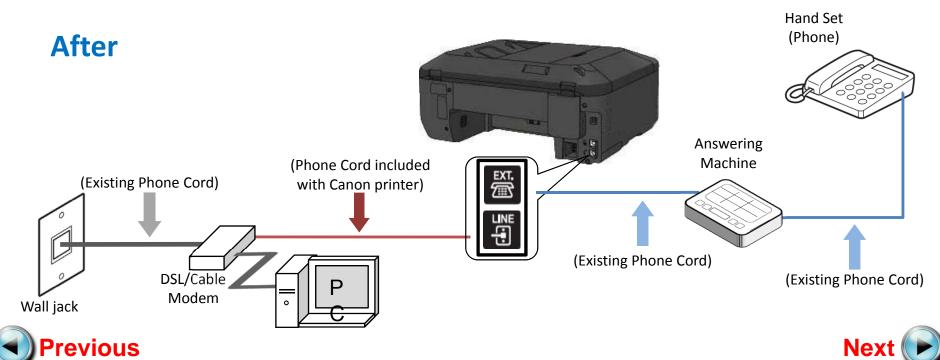
Plug the provided phone cord into the DSL/Cable Modem.
