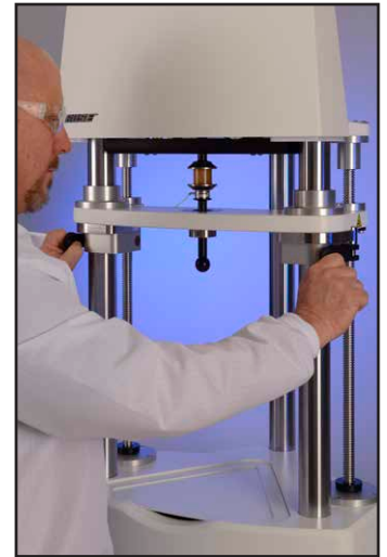
Figure 2 - Custom test fixture used for QA testing of Bose® passive radiator materials used in SoundLink® and SoundLink Mini portable Bluetooth® speaker products on Bose ElectroForce® 3220 test instrument.
