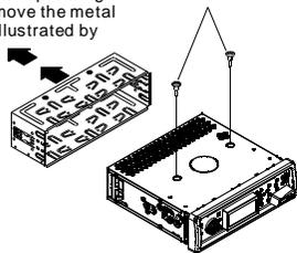
Remove the two screws that protect the CD player during transportation before operating the player.
