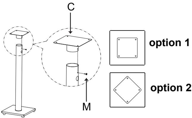
3. Insert top mount (C) into main pipe, fix it with screw (M).
