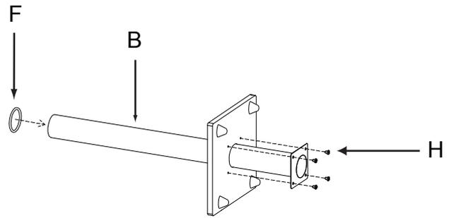
2. Insert main pipe (B) through the hole of base (A) and rubber ring (F), then fix it with screws (H).
