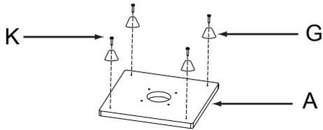
1. Fix feet (G) to underside of base (A) with screws (K).
