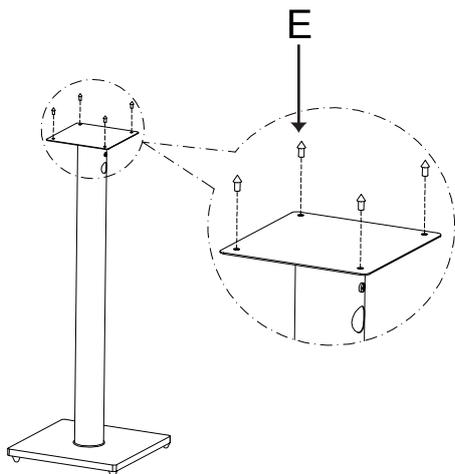
5. Insert metal studs (E) into the holes, speaker will rest on metal studs.
