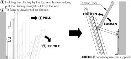
Tension Tool to adjust the tension in the tilt mechanism.
