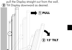
TIP: To push Display back against the wall, pull bottom edge outwards then push Display backwards.
