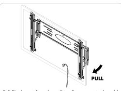
Pull Display out from the wall to allow access to the cable ports on the back of the panel.
