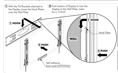
**OPTIONAL:** For larger screens, fix the protective self-adhesive foam pad (supplied) to the back of the panel. Position on the bottom edge, where the Display touches the wall.
