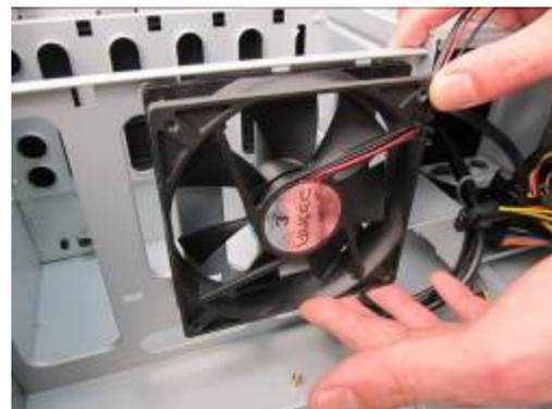
1. Find the fan mounting screw holes on the interior of the case. They are located on the interior of the internal 3.5" drive bay rails, below the cable management compartment.
