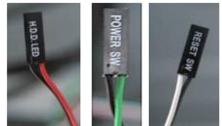
**Tip:** Polarity (positive and negative) does not matter for switches.
