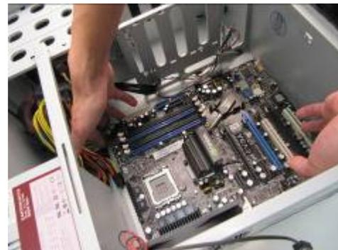
**Caution:** Make sure to remove any unused motherboard standoffs. They may come into contact with the back of the motherboard and may electrify your case exterior if left connected.
