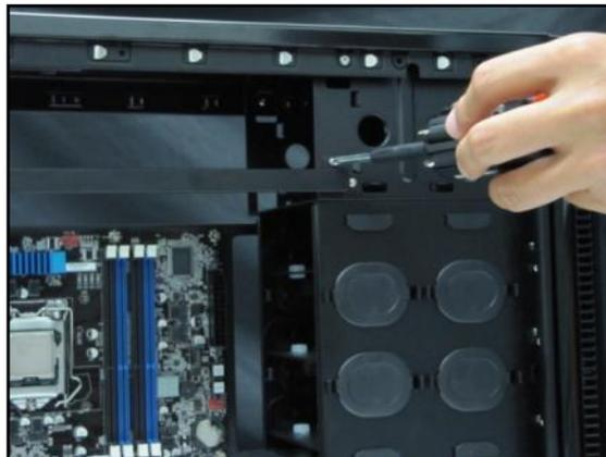
2. Remove the second screw with your other hand supporting the beam so the beam won't drop.
