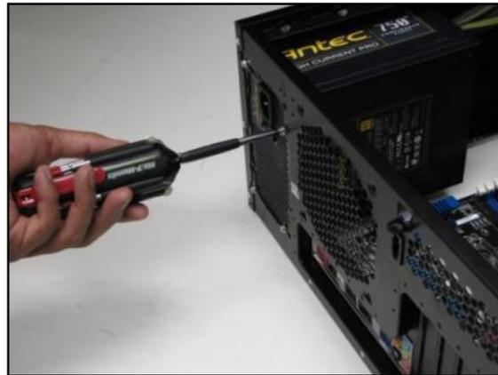
5. Re-attach the PSU support beam.
