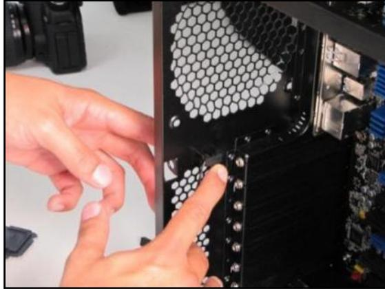
3. Preparing the KUHLER H<sub>2</sub>O backplate is specific to your CPU socket. Please refer to the KUHLER H<sub>2</sub>O installation guide, available at [http://www.antec.com/Believe\\_it/product.php?id=Mjc2OCYxNw==](http://www.antec.com/Believe_it/product.php?id=Mjc2OCYxNw==) (KUHLER H<sub>2</sub>O 620) or [http://www.antec.com/Believe\\_it/product.php?id=NzA0MzcwJjE3](http://www.antec.com/Believe_it/product.php?id=NzA0MzcwJjE3) (KUHLER H<sub>2</sub>O 920) for more information.
