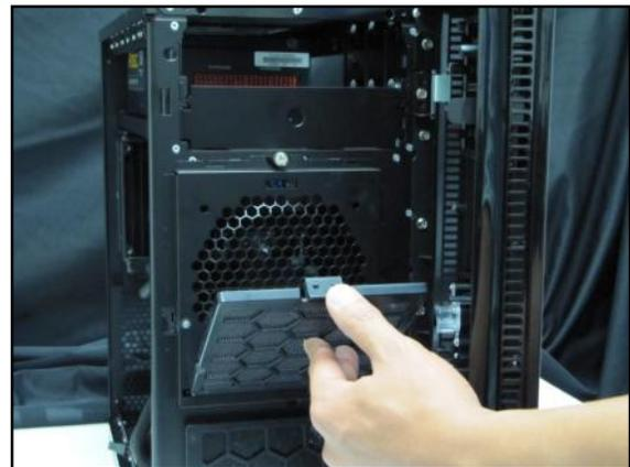
To clean the filter: Open the front bezel and locate the filter tabs. Push down on the tab and pull the filter away from the case to completely remove it.
