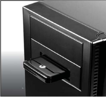
Ultimate flexibility: hot-swap drive bay compatible with Seagate® GoFlex® drives and SSDs, along with two front panel USB 3.0 ports.
