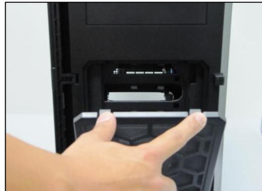
The P280 features a removable PSU filter that can be unlocked for maintenance and locked for transport. To remove the PSU filter, push the ends of the filter down then pull the filter toward you using the tab outside the chassis. You can also lock the filter by pushing up on the tab (once the filter is completely inside the chassis).
