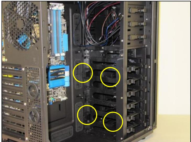
*Align your fan with the pegs that correspond with the fan screw holes on the fan.*
