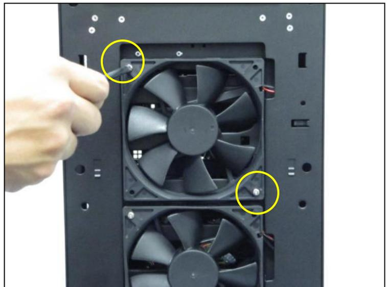
*Be sure to screw in the fan in the top-left and lower-right holes first.*
