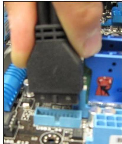
***Align the connector properly to prevent damage to your motherboard.***
