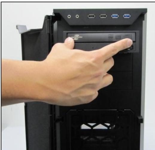
*Slide your 5.25" drive through the front chassis until it lines up flush with the front bezel.*
