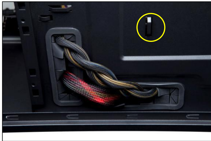
Use the grommet-lined cable routing holes to route PSU cables. The yellow circle shows a cable tiedown.
