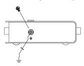
2. Make sure that the computer that the CE770L connects to and the monitor that the CE770RQ connects to are properly grounded.
