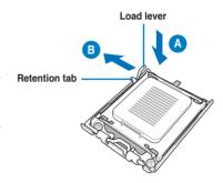
Lift the load lever in the direction of the arrow.
