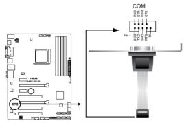
A88X-PLUS Serial port (COM) connector
