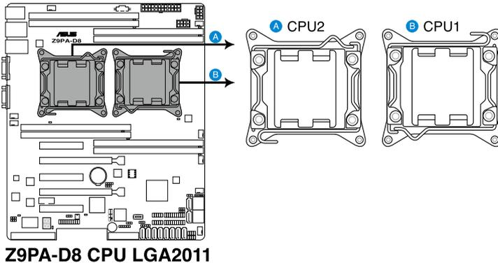
2. Press the left load lever with your thumb (A), then move it to the left (B) until it is released from the retention tab.
