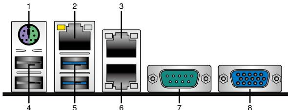
1. **PS/2 keyboard/mouse port.** This port is for a PS/2 mouse or keyboard.
