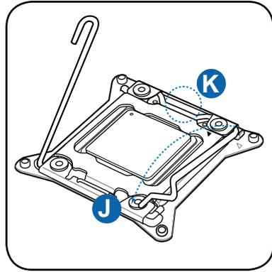
9. Insert the right load lever under the retention tab.
