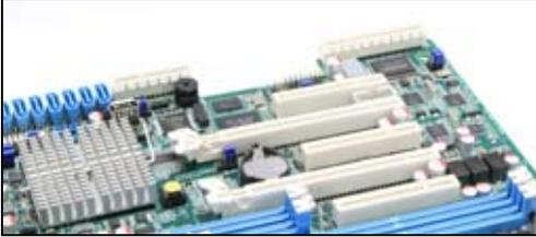
2. Align the golden fingers of the PIKE RAID card with the PIKE RAID card slot. Insert the PIKE RAID card into the PIKE RAID card slot. Ensure that it is completely seated on the PIKE RAID card slot.
