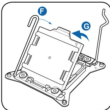
6. Position the CPU over the socket, ensuring that the triangle mark is on the top-right corner of the socket.
