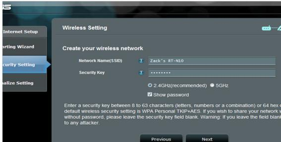
Assign a new SSID and password to the EA-N66. Enter a unique SSID to avoid any network issues.
