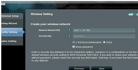
Assign a new SSID and password to the EA-N66. Enter a unique SSID to avoid any network issues.
