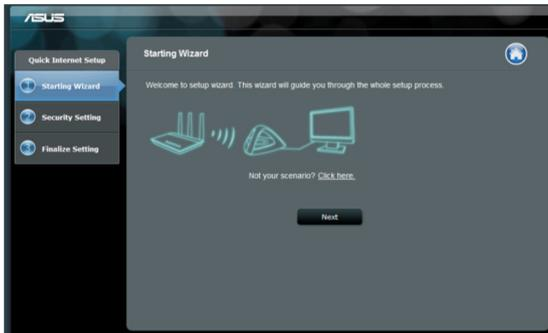
To set up Wireless Range Extender mode, do not click **Next** on the first page of Quick Internet Setup. Instead, click the link provided to switch setup mode.
