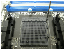
STEP 1: Lift Up The Socket Lever
