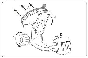
Step 3. Adjust the angle and rotation of the pedestal head by loosening the swivel-tightening ring (**D**).
