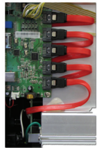
T5c mainboard (Port Multiplier Backplane)
