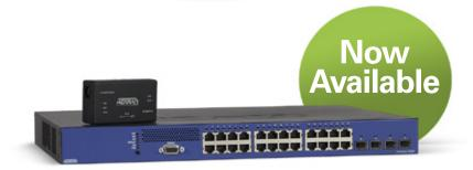
The NetVanta 1535P with ActivReach technology is the industry's only switch that can deliver voice, data, and PoE over legacy voice-grade cabling, as well as standard CAT5 cabling. The NetVanta 1535P is a managed, 28-port PoE, Layer 3 Lite, Gigabit Ethernet switch with ActivReach technology designed for fast, secure, cost-effective Local Area Network (LAN) switching.
