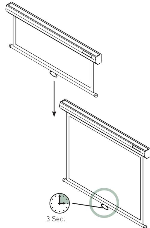
Retract the screen by pulling down the handle and then let go of it. The screen will retract into the casing.
