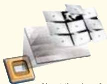
About the size of a postage stamp, the DLP chip is covered with tiny mirrors.
