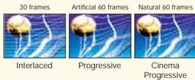
Powered by Samsung's Cinema Smooth technology, 3:2 Pull Down corrects for the artificial frames created when films are converted to DVDs. The result is a clearer image without the subtle motion artifacts caused by 24-to-30 frames per second video conversion.
