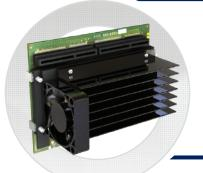
5A Dual Core Processor Board Processor/Socket: Dual-core 64-bit 3400e Speed: 1.8GHz Memory: 2GB DDR2 L2 Cache: 1MB Power: 20 Watts
