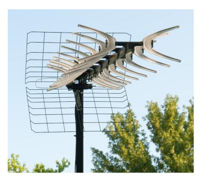
The 91XG is one of the highest gain UHF antennas made. This high performance UHF antenna has a higher gain and a smaller beam angle than conventional Yagi antennas. The reflector grids create and improved front to back ratio with shorter construction while the 91 elements truly make it one of the highest gain UHF antennas available.
