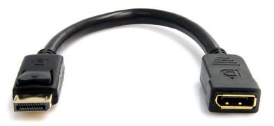
The DPEXTAA6IN 6-inch DisplayPort Port Saver Cable/coupler avoids expensive repairs to a computer or display. It does this by extending the port by 6in, thereby eliminating the weight and stress that would typically be placed on the port by a DisplayPort cable. This is especially useful in an environment where cables are unplugged and re-inserted frequently.
