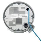
Only a single Ethernet cable is needed to connect the IK-WR14A to the network and electrical power
