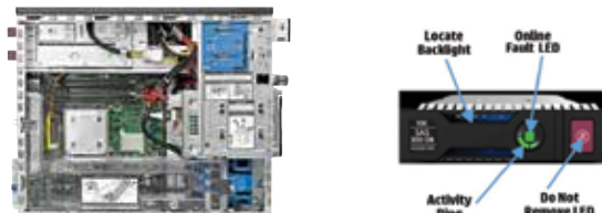
Figure 2. HP ProLiant ML310e Gen8 v2 Server: flexible configurations and easy serviceability, with tool-less access to all customer-serviceable system components
