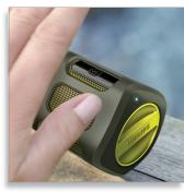
SHOQBOX is equipped with a motion senor. Simply swipe over the sensor from left to right or right to left, to skip to the next or last track. Put your hand over the sensor for a second to pause the music. Do it again to put it back on. Easy gesture control allows you to control your music the simplest way.
