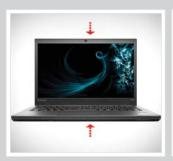
Rugged and Shock Resistant Light weight carbon fiber top cover with magnesium bottom shell and integrated roll cage
