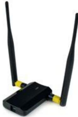
The USB300WN2X2D dual-band Wireless-N USB Network Adapter allows a USB-enabled computer to connect to a WiFi network on the 2.4GHz or 5GHz frequency. The adapter can be used for connecting to Wireless-A, B, G or N networks, and features dual 5dBi high gain antennas, as well as powered amplifiers to ensure optimized reception capable of supporting up to 300Mbps of data bandwidth over distances up to 3 times greater than a standard WiFi adapter.
