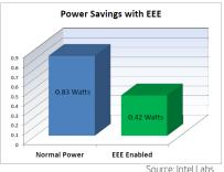
Energy Efficient Ethernet reduces the controller power to approximately 50% of its normal operating level.
