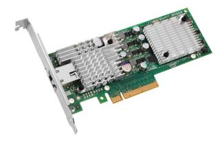
MSI-X enables more efficient response times and application performance. CPU utilization can be lowered further through stateless offloads such as TCP segmentation offload, header replications/splitting, and Direct Cache Access (DCA).
