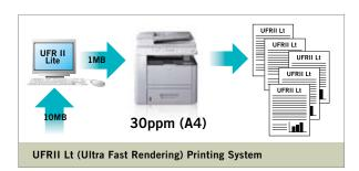
Not a fan of long print queues? You'll love Canon's in-built UFRII LT (Ultra Fast Rendering) printing system as you won't have to rely on your printer alone to do all the jobs. It enables integration between your computer and the printer's RAM for simultaneous job processing, balancing the workload and speeding up the printing process. The result? Quick First Print (QFP) of approximately 8 seconds, less downtime, and no expensive RAM upgrades required.
