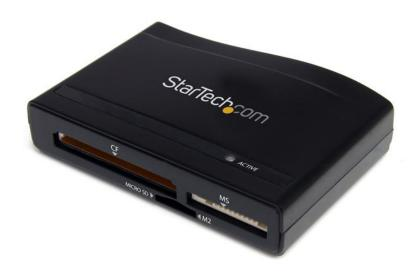
The FCREADHCU3 USB 3.0 Card Reader enables easy read/write access to a variety of popular flash memory card formats/types (CompactFlash®, Secure Digital®, Memory Stick®) in a single unit, over a high speed USB 3.0 connection.
