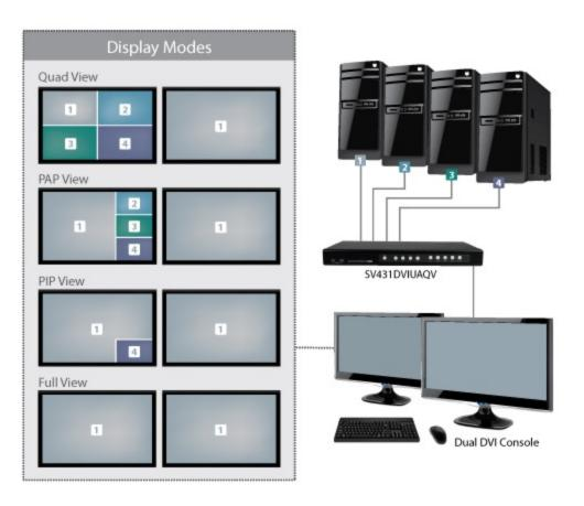
The KVM switch integrates front, push-button controls for simple switching between PCs, choosing your desired display mode and accessing the KVM menu, plus hot-keys and RS-232 command support, for flexible control.
