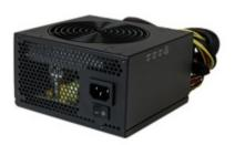
The ATX2PW450BR 450 Watt 80 Plus® Bronze Power Supply offers an energy efficient replacement or upgrade for powering your desktop PC. Operating at an 82% to 85% efficiency between 20% and 100% load, 80 Plus Bronze power supplies deliver a significant improvement over standard-efficiency power supplies that helps reduce energy consumption and cost of operation.
