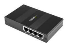
The ST124UTPE 4 Port VGA Video Extender over Cat 5 (UTPE Series) allows up to 5 (1 local and 4 remote) monitors to be connected to a single VGA source.
