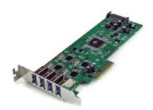
The PEXUSB3S400 PCI Express USB 3.0 Card adds 4 independent external USB 3.0 ports to any PCI Express x4-enabled computer system, with full bandwidth support (up to 5Gbps) per port when connected to USB 3.0 devices. Unlike other USB 3.0 cards, which share the maximum bandwidth between multiple ports, the PEXUSB3S400 offers maximum transfer rates to each device when multiple devices are connected.
