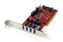
The PCIUSB3S4 4-Port PCI to USB 3.0 Card enables legacy PCI slots to support the SuperSpeed USB 3.0 standard, which is capable of data transfer rates up to 5 Gbps. Using USB 3.0 devices with this card will increase data transfer rates with up to 1.3 Gbps of available bandwidth (PCI bus limit) - more than doubling performance compared to a USB 2.0 connection.
