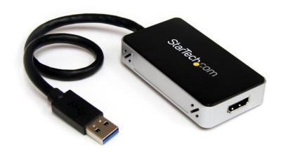
The USB32HDE USB 3.0 to HDMI® Adapter turns an available USB 3.0 port into an HDMI output, with high resolution 1920x1080 (1080p) video support - a convenient external video solution that makes it easy to add multi-monitor capability to a USB 3.0-enabled desktop or laptop computer (optimal performance from USB 3.0, backward compatible with USB 2.0).
