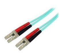
The A50FBLCLC10 10m 850nm Laser-Optimized Multimode Fiber (LOMMF) Aqua Cord features 50/125 micron fiber for high-speed, high bandwidth data transmissions over 10 Gigabit Ethernet and Fiber Channel networks - the perfect solution for fiber cable runs between multiple backbone switches, hubs and routers as well as higher end networking equipment.
