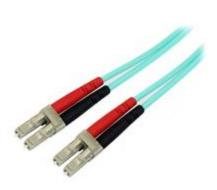
The A50FBLCLC3 3m 850nm Laser-Optimized Multimode Fiber (LOMMF) Aqua Cord features 50/125 micron fiber for high-speed, high bandwidth data transmissions over 10 Gigabit Ethernet and Fiber Channel networks - the perfect solution for fiber cable runs between multiple backbone switches, hubs and routers as well as higher end networking equipment.
