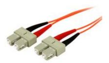
The 50FIBPSCSC5 5m SC to SC Plenum Fiber Cable features 50/125 micron fiber for high-speed, high bandwidth data transmissions over Gigabit Ethernet and Fiber Channel networks, with support for duplex multimode applications.
