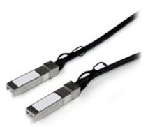
The SFPCMM1M Cisco Compatible 1m SFP+ cable is a fully hot pluggable, direct attach cable, supporting 10 Gigabit Ethernet and Fiber Channel applications connected through (Small Form Factor Pluggable) SFP+ ports.
