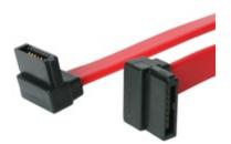
The SATARA12 Right Angle (90-degree) SATA cable (12in) enables you to plug in your SATA hard drive in hard to reach areas or tight spaces, using right-angled SATA connectors to reduce the amount of space required at the connection point and supports full SATA 3.0 bandwidth of up to 6Gbps when used with SATA 3.0 compliant drives.
