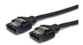
The LSATARND6 6-inch latching round SATA cable is a high quality SATA 6Gbps cable that features a rounded design to help improve airflow inside a computer or server case by providing less resistance as air passes around the cable, in turn helping to ensure optimal cooling for optimized system performance.
