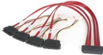
The SAS8482P50 SFF-8484 to 4x SFF-8482 SAS cable features one 32-pin SFF-8484 receptacle which fans out to four 29-pin SFF-8482 receptacles with LP4 power supply connectors, providing a reliable solution for connecting up to four SAS HDDs to a SAS controller or backplane.
