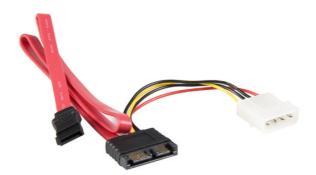
StarTech.com's Slimline SATA Male to SATA with LP4 Power Cable Adapter features one SATA (7-pin) female data connection and one LP4 power connection on one end, and a slimline Serial ATA male connection on the other - allowing you to connect a drive with a female slimline SATA port to a computer motherboard that does not have a slimline connection available.
