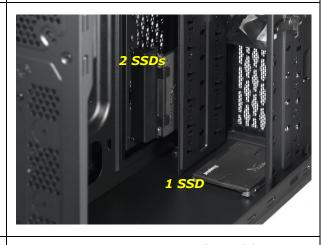
Supports up to 3 SSDs – 2 on the tool-less cage, 1 at the bottom of HDD cage
