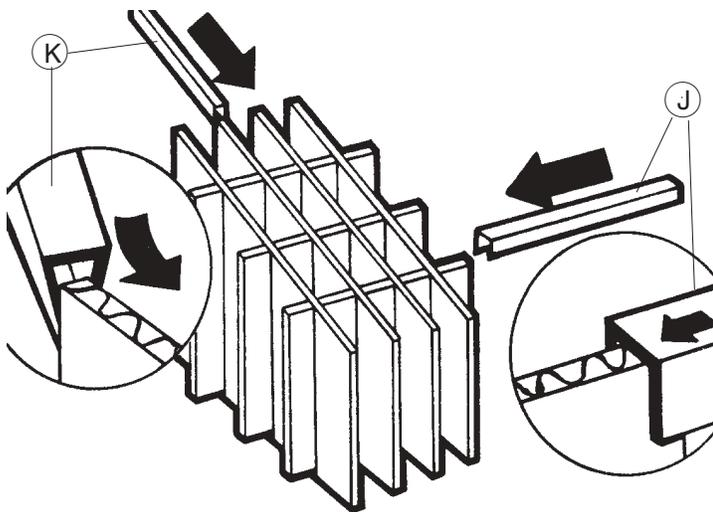
**6** Place the assembled divider into the shell.
