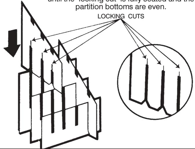
**5** Slide the (J) Open Channels over the RECTANGULAR partitions; then slide the (K) Closed Channels over the triangular partitions.
